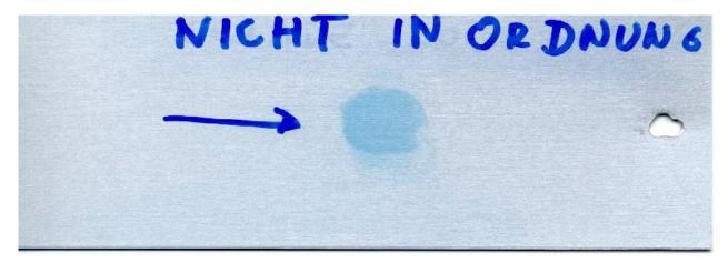
A sample section, which has been treated with a drop of the acid solution before being subjected to the test solution and carefully rinsed with deionised water, can be used as a reference for an "openly porous" oxide layer.
