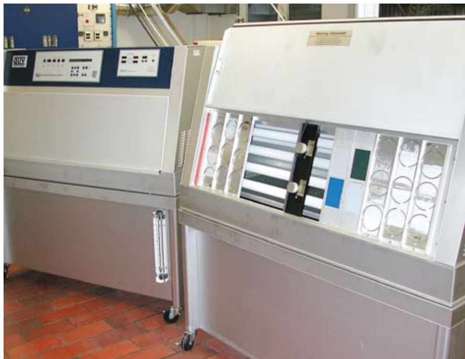
Laboratory test in accordance with DIN EN ISO 11507, QUV-B 313, Cycle: 4h Humid, T = 40°C, 4h Dry, T = 50°C Level of radiation: 0,75 W/m 2
