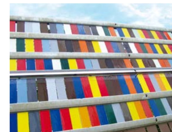
To assess weatherproofing coated samples are exposed in Florida for up to 5 years.
