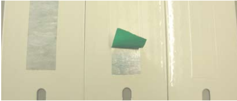
Picture 1 – taped sample sheets to avoid scarring
