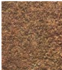
Steel surface with tinder that has either rusted away completely or can be scraped off, yet only showing few signs or rust that is visible to the naked eye
