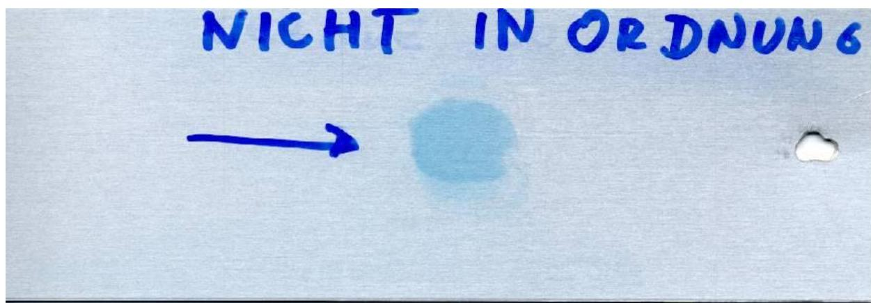
A sample section, which has been treated with a drop of the acid solution before being subjected to the test solution and carefully rinsed with deionised water, can be used as a reference for an “openly porous” oxide layer.
