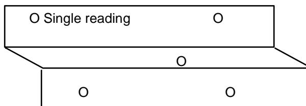
If a measuring point displays less than 80% of the prescribed coating thickness, then the sample must be rejected and assigned to column 3 in the table in XYZ.
