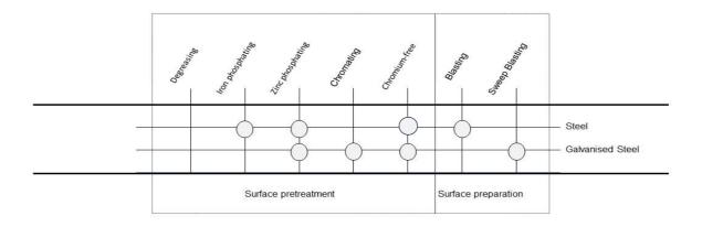
Galvanised components with a chromate layer as temporary corrosion protection are pre-treated based on EN 12487. In this case, ensure that the temporary corrosion protection is removed without any residue. This might have to be coordinated with the pre-treatment manufacturer.
