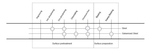
Galvanised components with a chromate layer as temporary corrosion protection are pre-treated based on EN 12487. In this case, ensure that the temporary corrosion protection is removed without any residue. This might have to be coordinated with the pre-treatment manufacturer.
